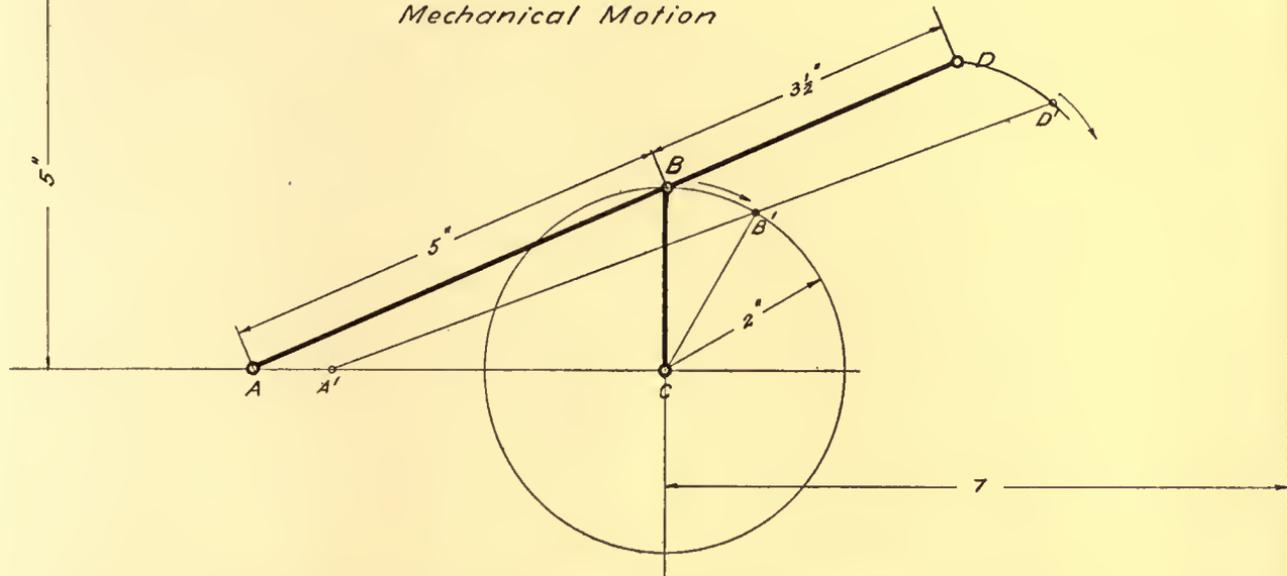
*Path of motion of point D during one revolution of B around centre C.
