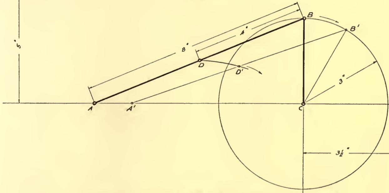
*Path of motion of point D during one revolution around centre C
