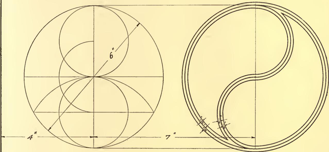
*Note: Show construction in fine lines on left side of plate as above; omit dimensions.*
