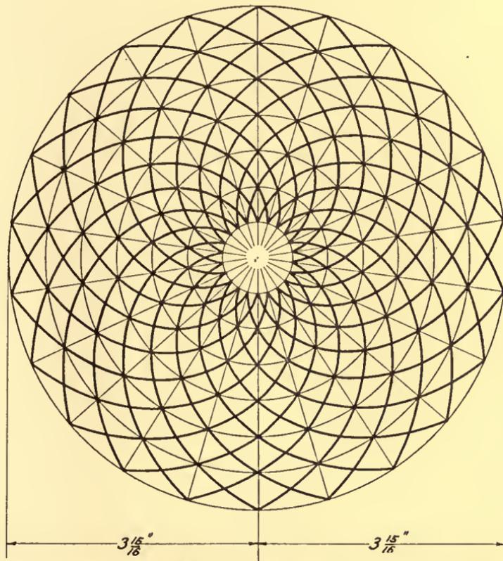
*Note: Omit dimensions, but provide construction in fine red lines. For construction divide radius into 7 and circumference into 22 equal parts.*
