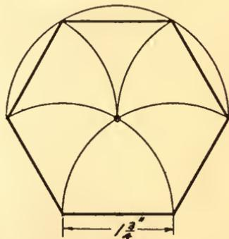
To construct a hexagon on a given line.
