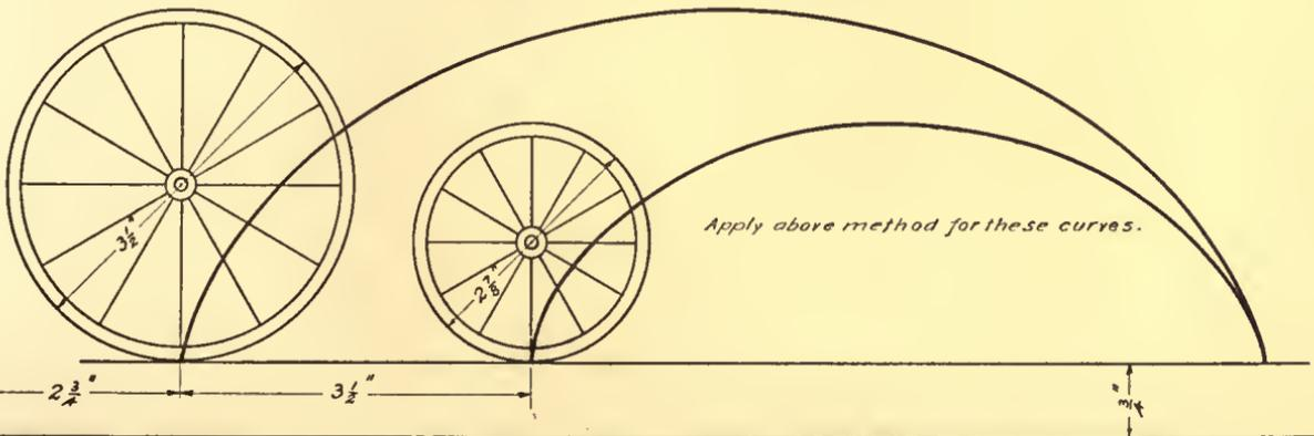
*Note: Omit dimensions, but provide construction of cycloid in fine red lines and numerals in black ink. Omit construction on Illustration of cycloid.*
