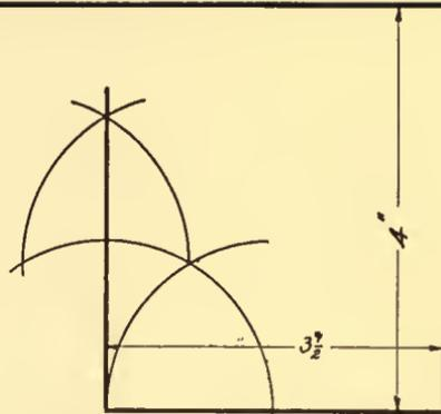
To draw a perpendicular at the end of a given line.
